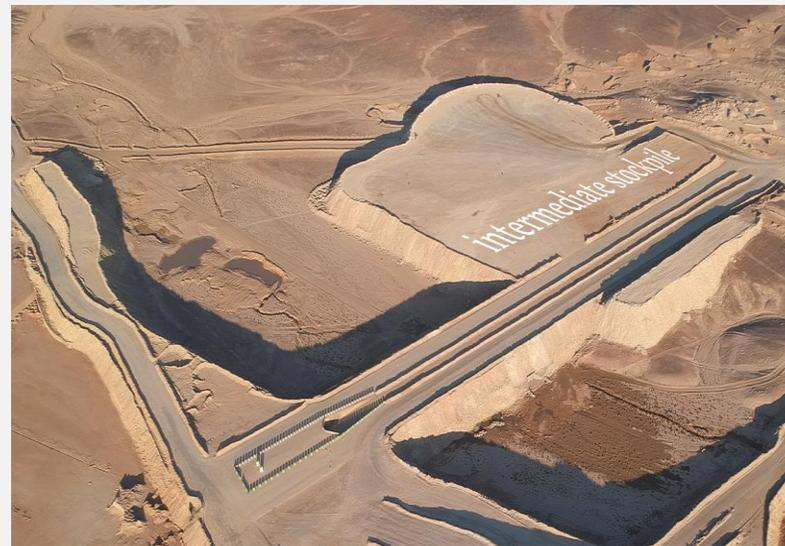
Figure (3): Dam bridge, Intermediate stockpile (north-east dumping area), and roads network.
