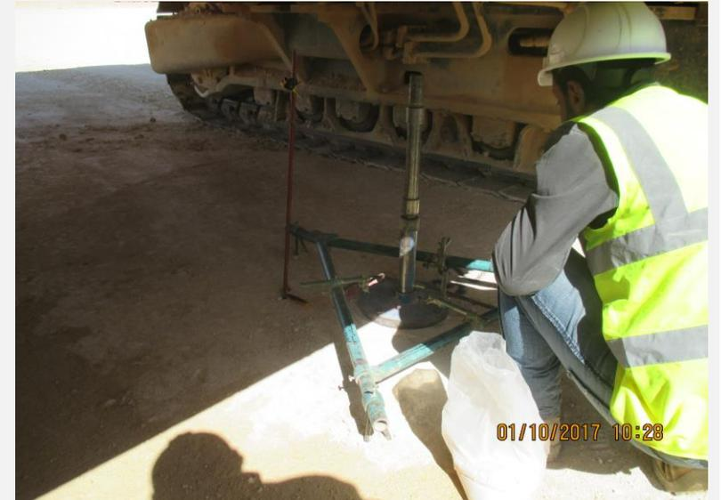
Plate bearing test
