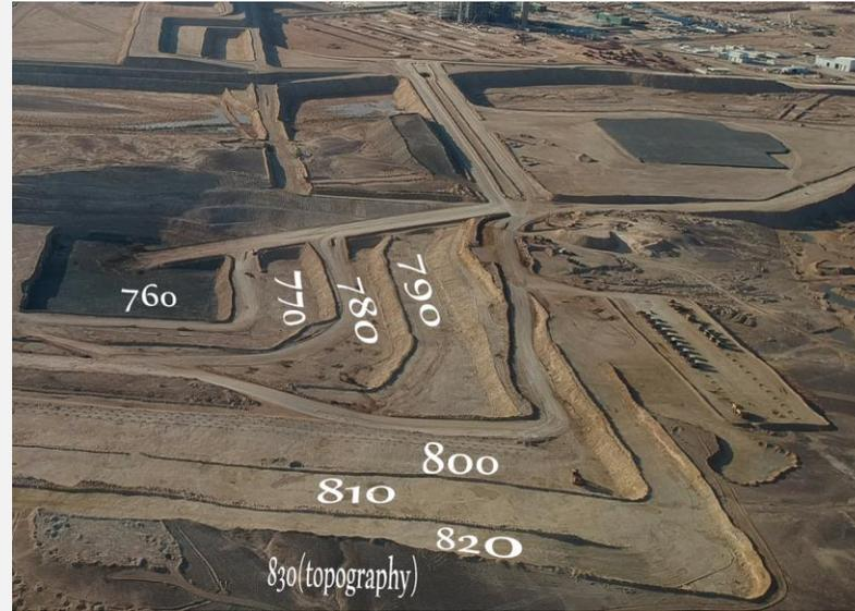
Figure (1): mine benches and it levels
